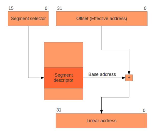
Figure 5.1: Translation of logical addresses to linear addresses.
