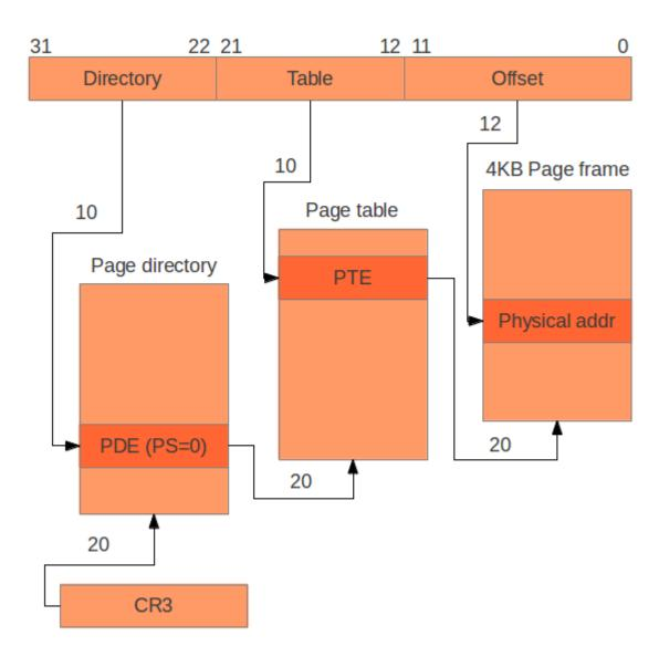
Figure 9.1: Translating virtual addresses (linear addresses) to physical addresses.
